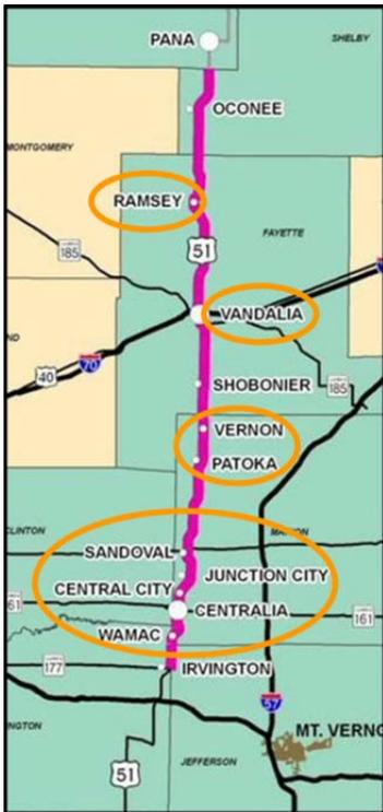
*Build Alternatives to the east, west, and through the larger towns circled above were developed. For the areas between towns, Build Alternative options included widening existing US 51 to the east side, west side, or along both sides.*
